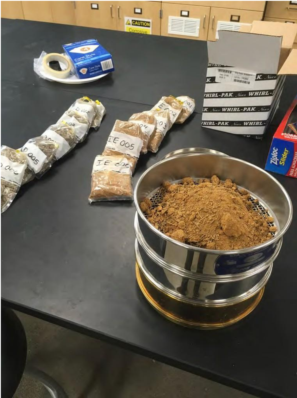
Figure 23: Samples being sieved to remove the larger than 2 mm fraction. Photo by Scott Kugel, November 2017.
