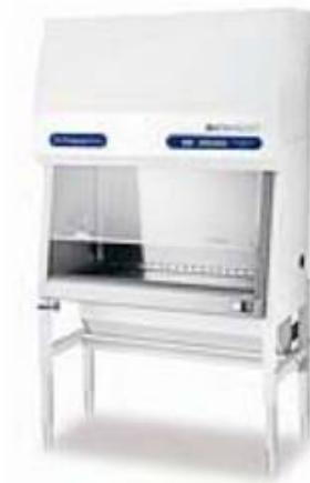
It is imperative that Class I and II biological safety cabinets be tested and certified at the time of installation within the laboratory, at any time the BSC is moved, and at least annually thereafter. As with any other piece of laboratory equipment, personnel must be trained in the proper use of the biological safety cabinets. Of particular note are activities that may disrupt the inward directional airflow and have been demonstrated to cause aerosolized particles to escape from the cabinet:
