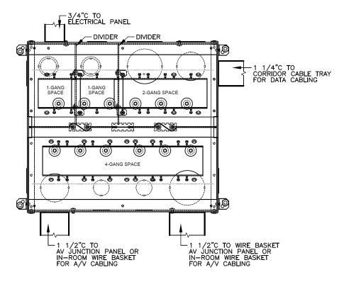
Some applications may require a high-capacity floor box, such as the FSR FL-600P-x. The Designer shall discuss with the AVM on a project-by-project basis about whether the larger floor box would be appropriate.
