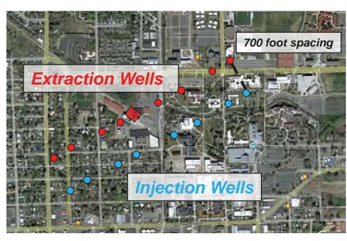
**NOTE:** Due to scale, wellfield design does not consider current or planned buildings or utilities. Design was developed with regard to well spacing and groundwater flow direction.
